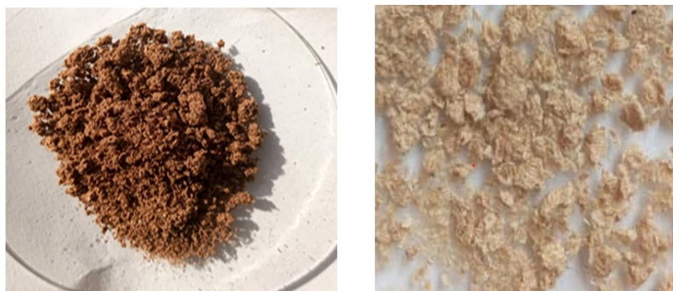
Fig.1 (a). Jackfruit peel cellulose after extraction. (b). Jackfruit peel cellulose after AHP bleaching
