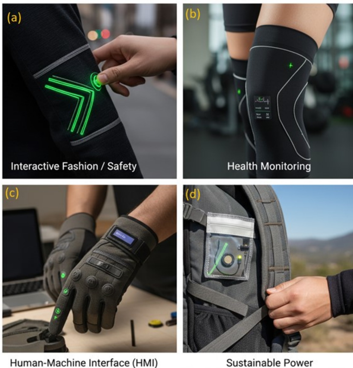
Figure 12. Applications of electroluminescent (EL) yarns in smart textiles. (Interactive Fashion and Safety: Apparel with EL yarns for illumination and visibility(a). Health Monitoring: Compression wear displaying physiological data(b). Human–Machine Interface (HMI): EL gloves providing tactile and visual feedback(c). Sustainable Power: Textile EL modules integrated with energy harvesting for self-powered use(d).
