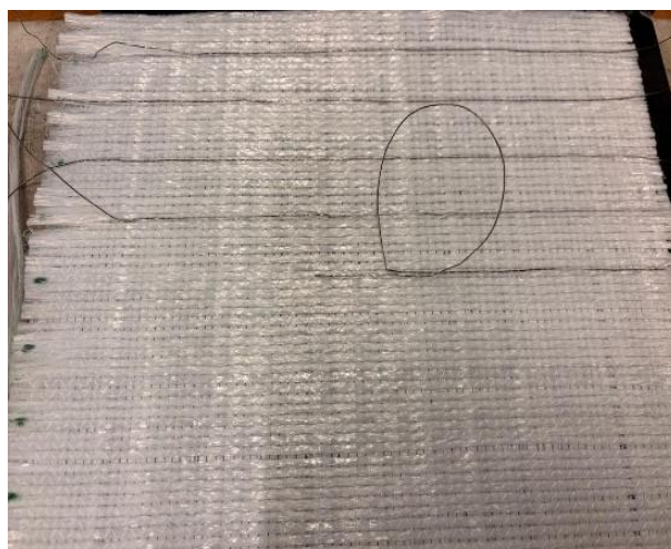
Figure 2. Fixation of the electrically conductive PEEK-MWCNT monofilament yarn with bonding threads to the GF/PP fabrics.
