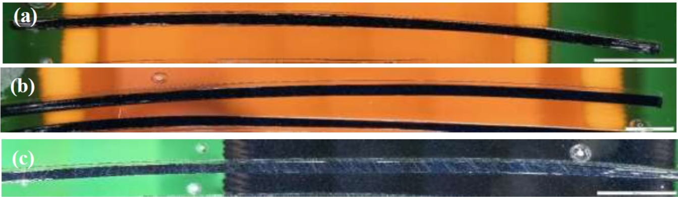
Figure 11. Influence of the take-off speed of (a) 90 m/min, (b) 100 m/min and (c) 110 m/min on the longitudinal view of the C-S filament yarns. with a 5 rpm TSE speed for the PEEK-MWCNT core and with a 5 rpm SSE speed for the PEEK sheath.
