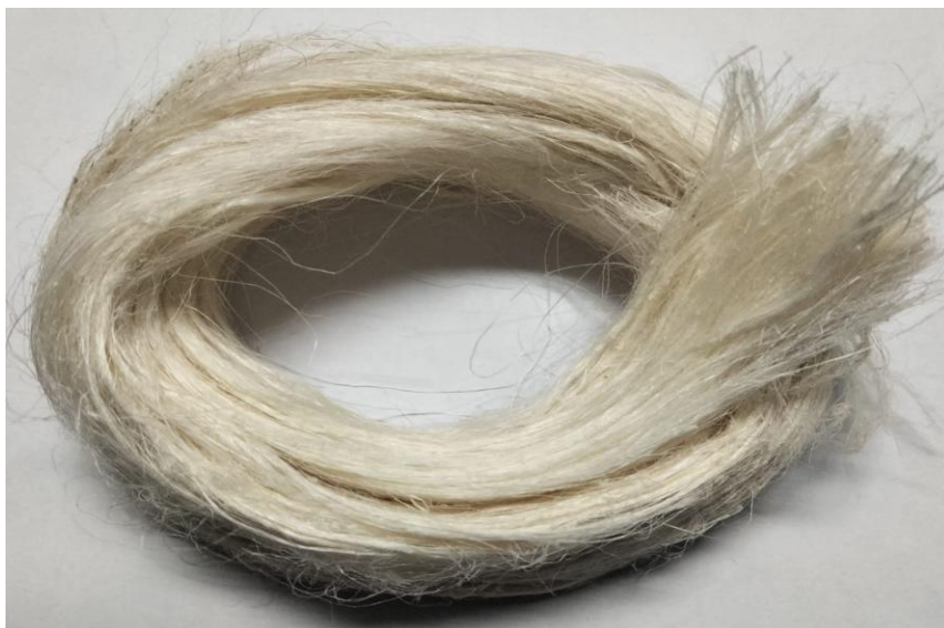
Figure 1: Long staple pineapple fiber.
